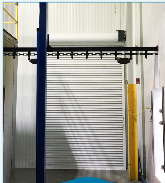
Overhead doors facilitate system maintenance and provide forklift access.
