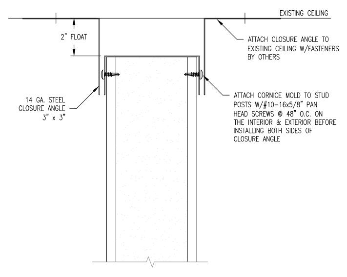
ABOVE DETAIL IS DESIGNED TO ALLOW THE EXISTING STRUCTURE TO DEFLECT WITHOUT BEARING ON PORTAFAB WALL. AS SUCH, DO NOT ATTACH CLOSURE ANGLE TO PORTAFAB WALL.
