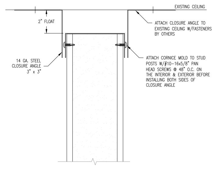
ABOVE DETAIL IS DESIGNED TO ALLOW THE EXISTING STRUCTURE TO DEFLECT WITHOUT BEARING ON PORTAFAB WALL. AS SUCH, DO NOT ATTACH CLOSURE ANGLE TO PORTAFAB WALL.
